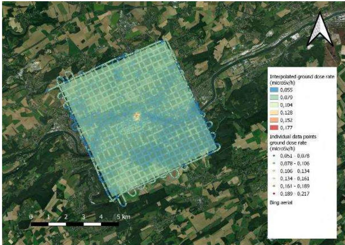
Figure 93: The dose rate in microSv per hour ( $\mu\text{Sv/h}$ ) on the ground determined from helicopter measurements after correction for height above ground above the CN Tihange and wider surroundings. The scale and colors are chosen to visualize small differences in the dose rate, e.g. you can very clearly recognize the course of the Meuse River, due to the lower natural radioactivity levels measured above water. A small increase is visible above CN Tihange: see also Figure 95 and text).
