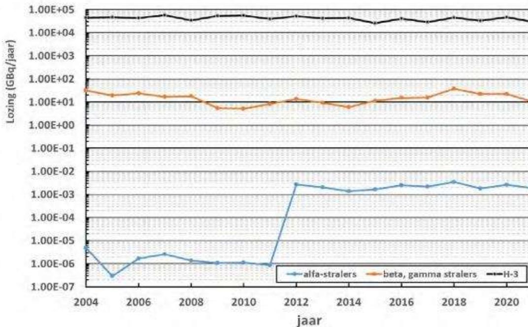
Figure 99: Evolution of liquid discharges from Tihange Nuclear Power Plant into the Meuse River for the period 2004-2021.<sup>lxvii</sup>
