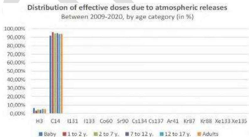
Figure 98: Distribution of effective dose in percent for the total dose impact of gaseous discharges by age group and by radionuclide discharged for the period 2009-2020<sup>lxviii</sup>.
