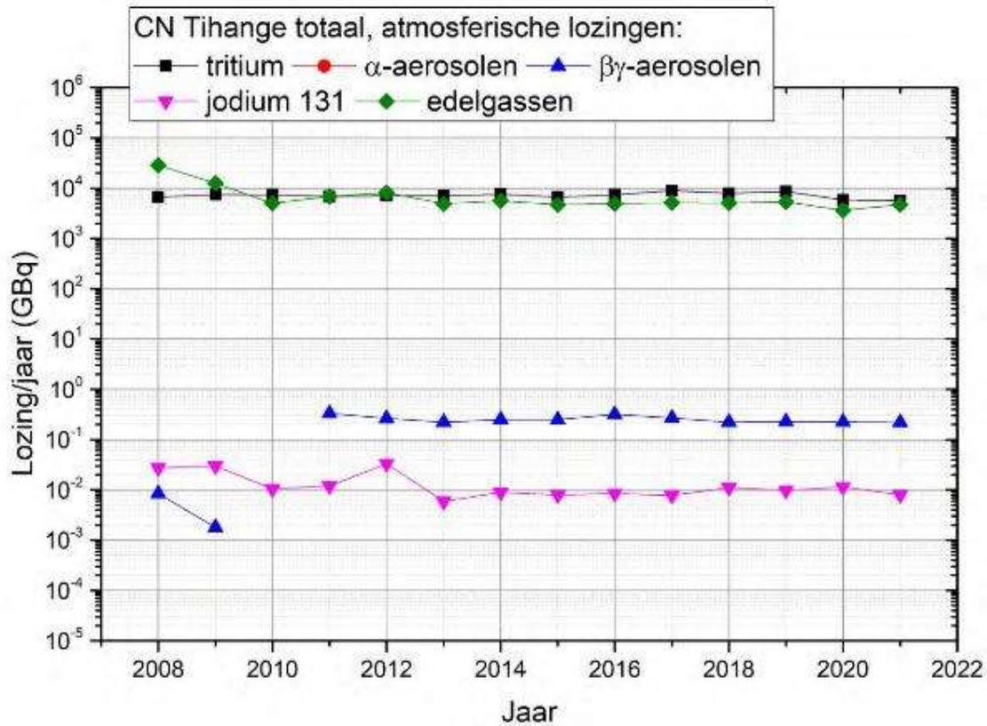
Figure 96: Gaseous discharges per year for the total CN Tihange<sup>134</sup> site.
