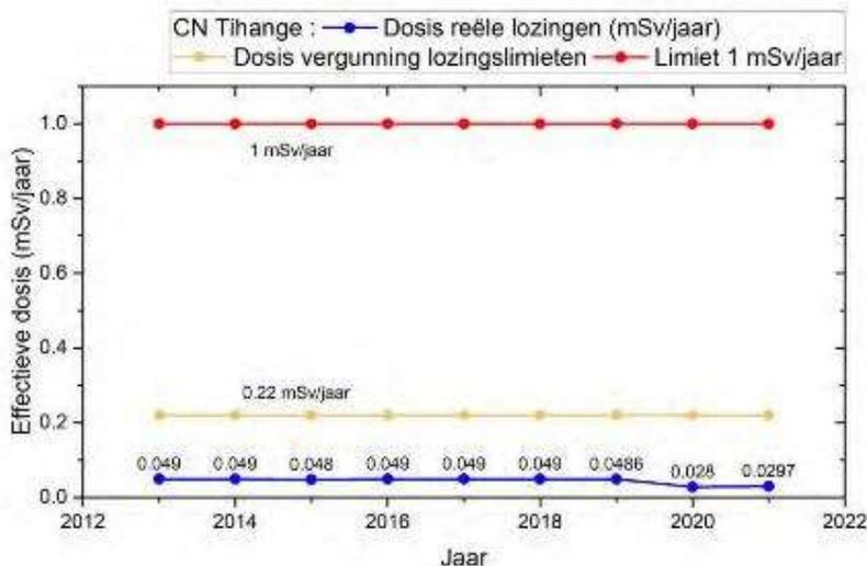
Figure 103: Effective dose for most critical individual in the vicinity of CN Tihange calculated from reported real discharges<sup>xxxvii</sup>. For comparison, the dose limit for the public is shown and the dose corresponding to the discharge limits.
