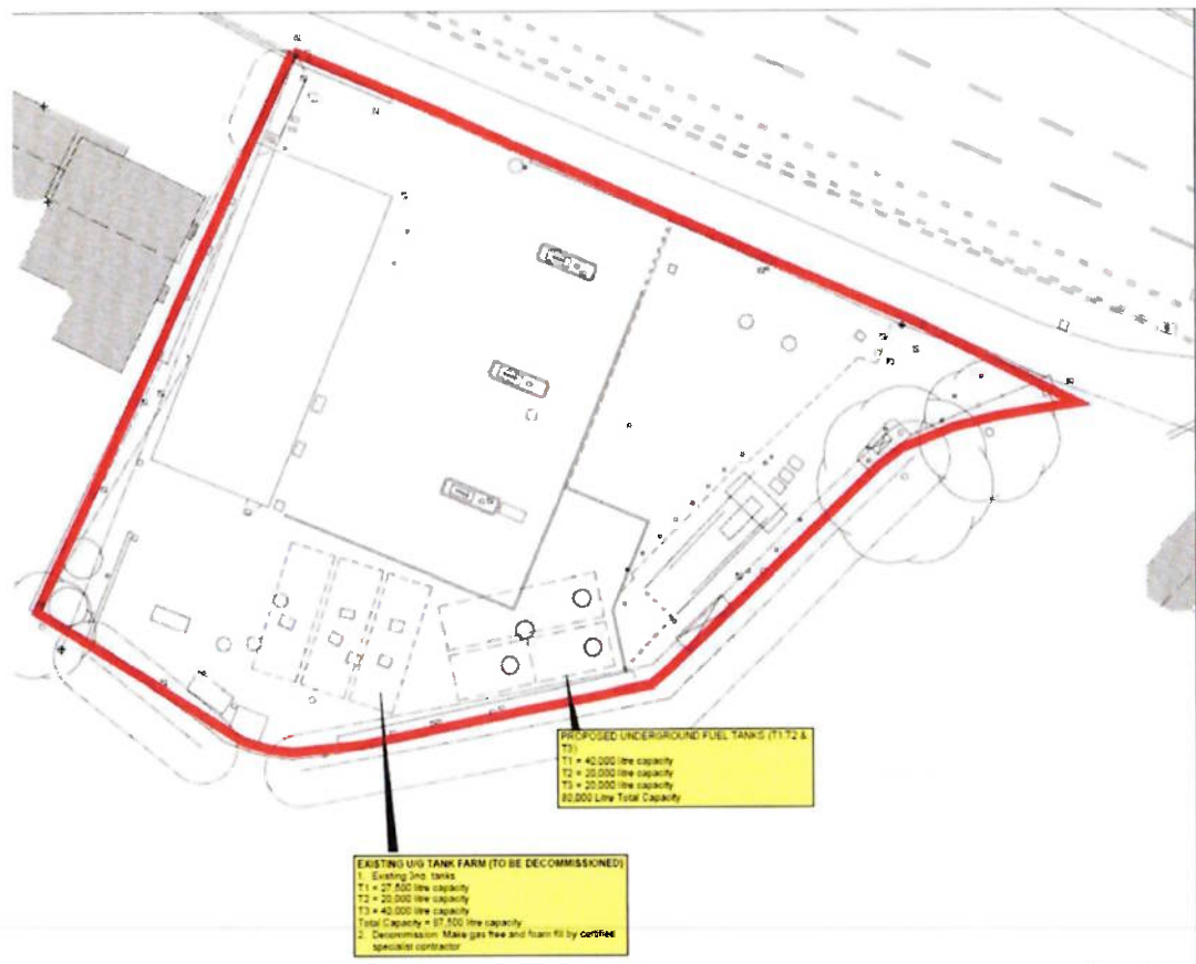
Fig No.6 Extract from site layout plan prepared by JA Gorman Consulting Engineers showing location of proposed new tanks (2 in total)
