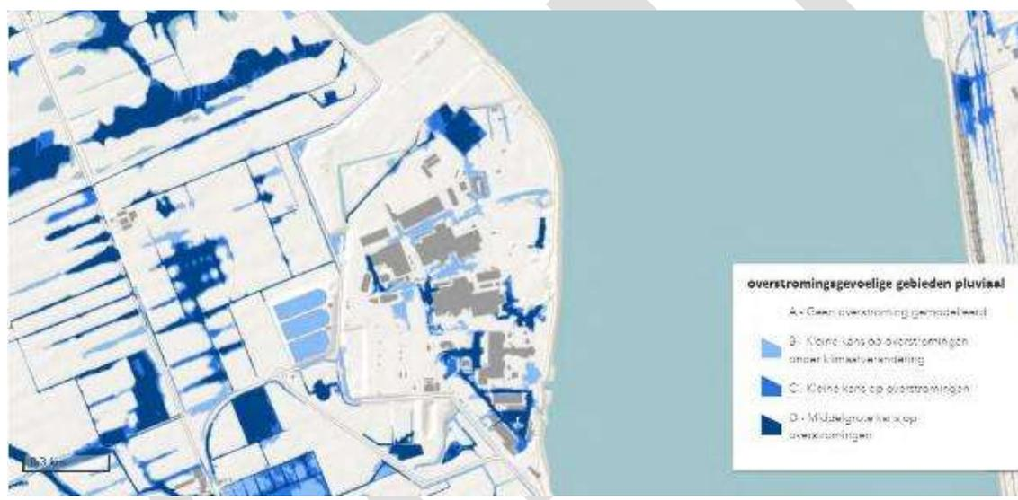
Figure 34: Pluvial flood prone areas (water assessment map, source: waterinfo.be).
