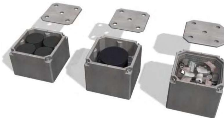
Figure 27: Illustrations of the three types of caissons<sup>svi</sup> containing waste: type I (left), type II (center) and type III (right).
