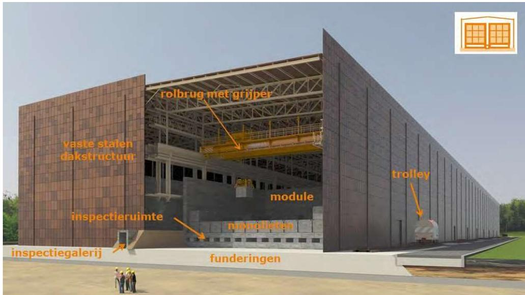
Figure 28: Sketch of the repository for category A waste during backfilling with <sup>monolithslvii</sup>.
