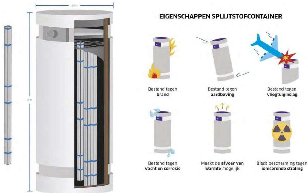
Figure 26: Principle of dry storage of spent fuel elements in Dual Purpose Casks (DPC) as provided in the  $SF_2$  storage facilities<sup>lii</sup>. The packaging consists of a metal structure designed to allow the residual heat of the spent fuel to be passively dissipated by internal conduction, radiation and natural convection. The package is made of metal and other materials that provide protection from ionizing radiation.
