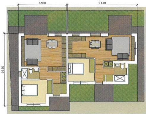
Floor Plan-Proposed Type 1 (scale 1:200)
