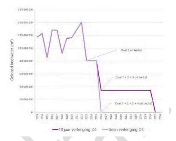
Figure 33: Volume of cooling water (m<sup>3</sup>) discharged as a result of the 10-year extension of operation of Doel 4 compared to the reference situation (no extension).
