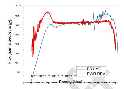
Figure 76: Normalized neutron spectrum per unit of lethargy.
