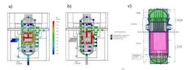
Figure 75: Schematic representation of (a) the simulated neutron flux in a reactor vessel, (b) the waste class classification derived from it, and (c) indication of the transition zone (in gray) for the a priori classification into category A (green) or B waste (purple). a) and b) taken from. lxxvi
