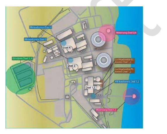
Figure 44: Cooling water principle diagram showing water capture Doel 1&2 and Doel 3&4 (Source: Electrabel nv, 2011).
