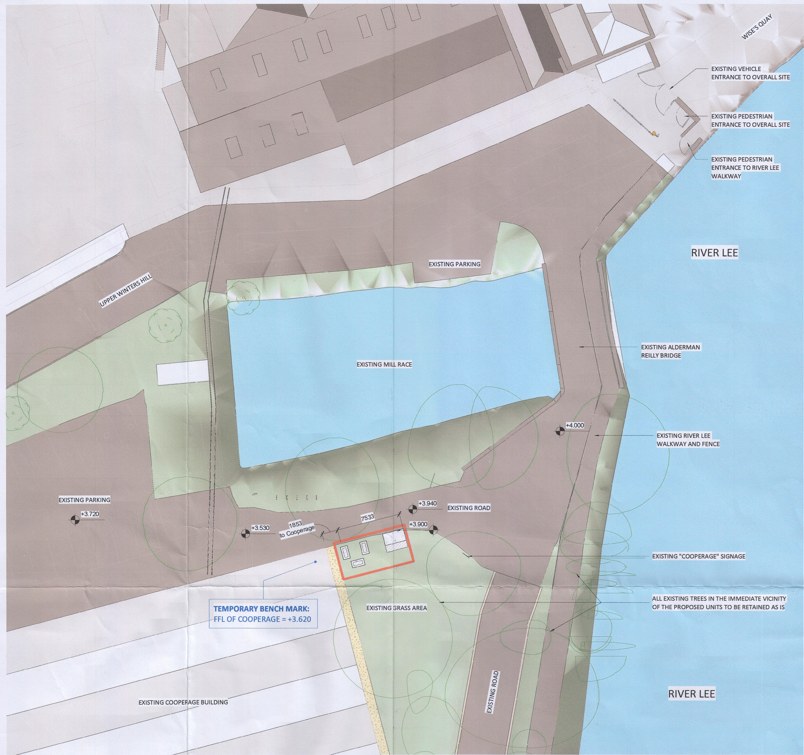
1 PLANNING SITE PLAN - ESB SUB UNIT AND ANCILLARIES SCALE: 1 : 250
